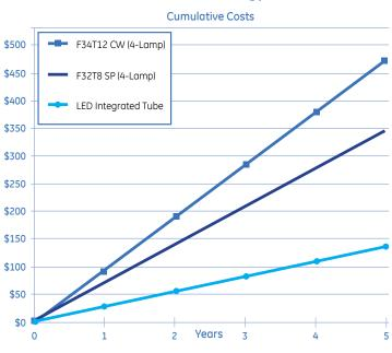
Savings calculations are based on energy costs using \$0.11 per kWh and 16 hours of daily operation.
